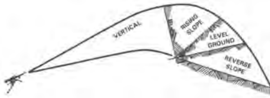
Figure 6-4. Effect of Ground Slopes on the Beaten Zone.
