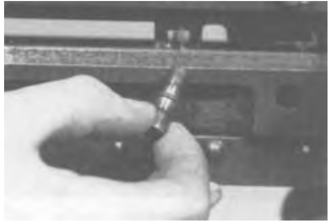
Figure 4-11. Removing the Bolt Stud.
