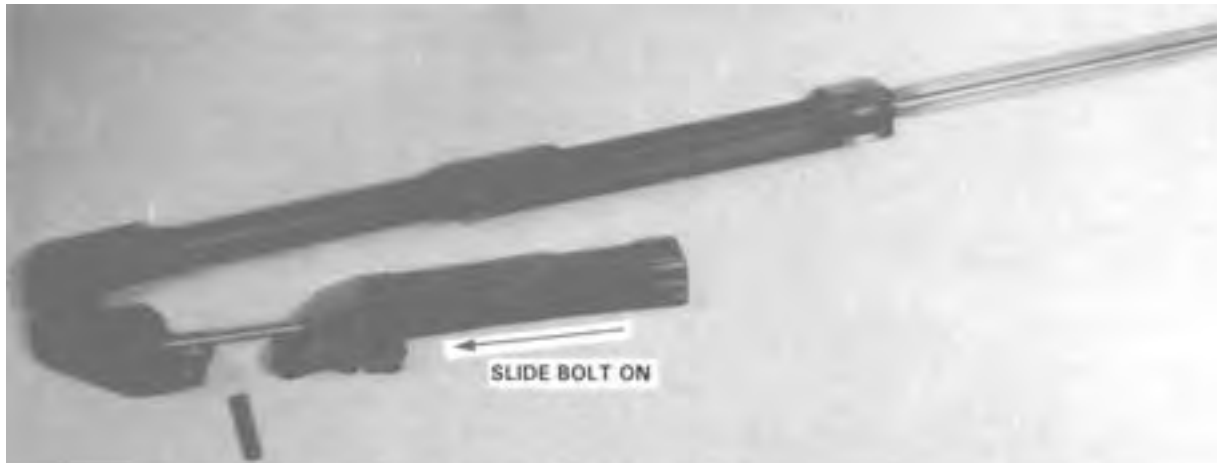
Step 1. Sliding the Bolt Over Firing Pin.
