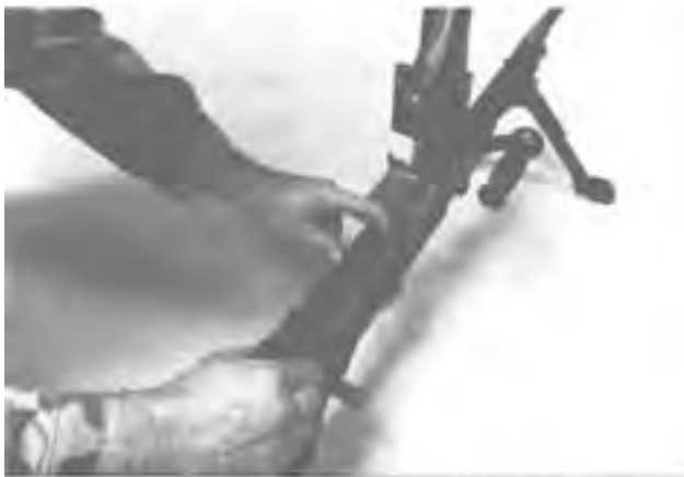
Step 2. Pushing Against the Face of the Bolt.
