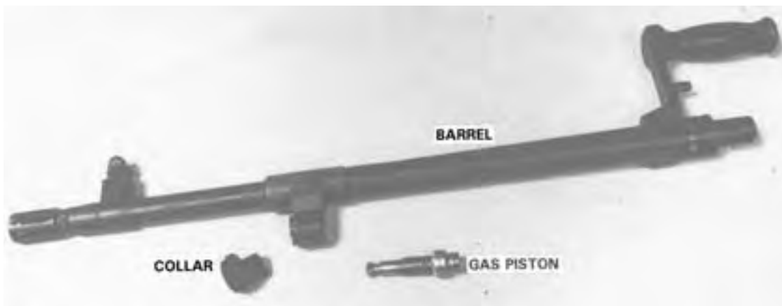
Figure 3-18. Barrel Group, Detailed Disassembly.
