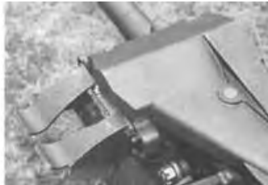
Figure 5-48. Attach Feed Throat to Feeder.
