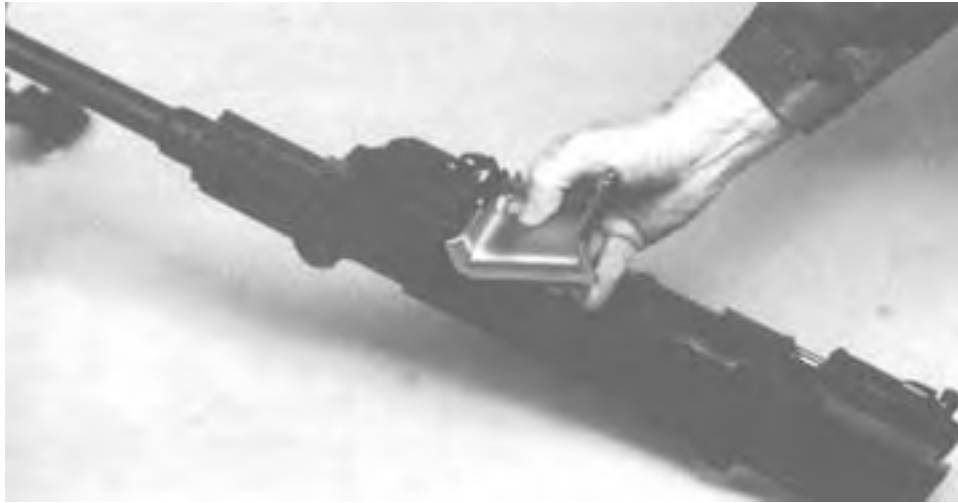
Figure 3-21. Aligning the Feed Tray Guides.
