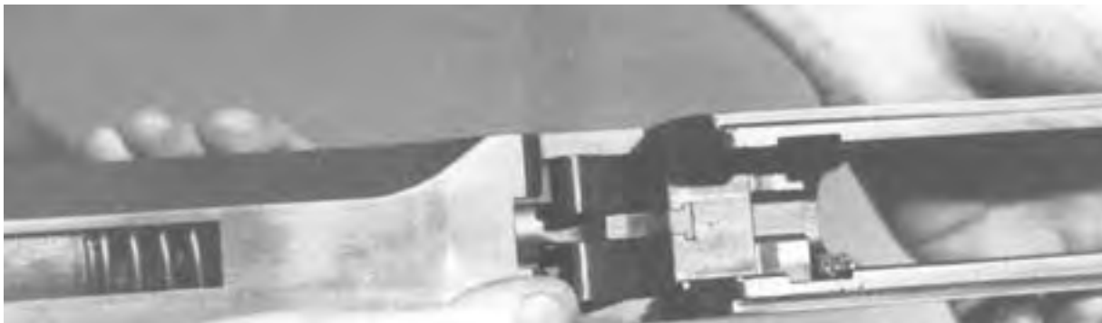
Figure 4-18. Joining the Barrel Extension Group and Barrel Buffer Group.
