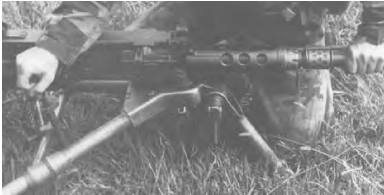
Figure 4-7. Removing the Barrel.
