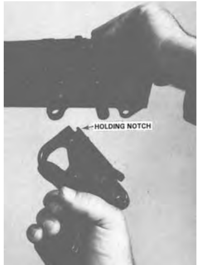
Figure 3-11. Replacing the Trigger Housing Group.
