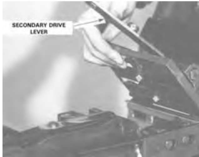
Figure 5-9. Removing the Secondary Drive Lever.
