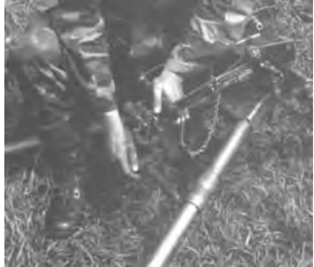
Figure 5-52. Attaching the T&E to the Tripod.
