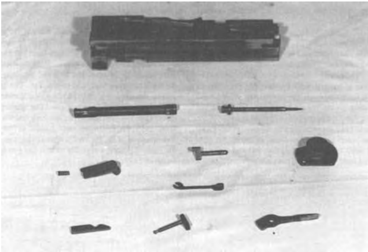
Figure 4-19. Bolt Group, Exploded View.
