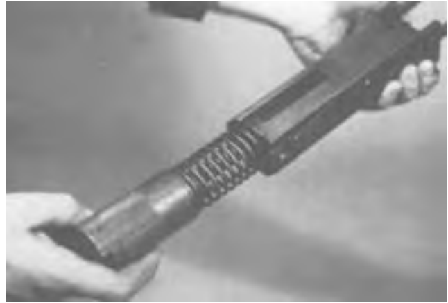
Figure 4-16. Separating the Barrel Buffer Assembly From the Barrel Buffer Body Group.
