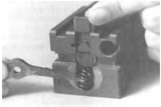
Figure 4-29. Removing and Replacing the Sear and Sear Spring.
