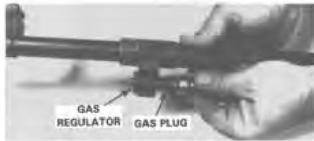
Step 3. Sliding Gas Plug Out of Gas Regulator.
