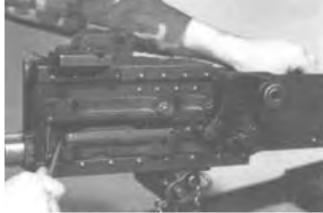
Figure 4-14. Removing the Barrel Buffer Group and Barrel Extension Group.
