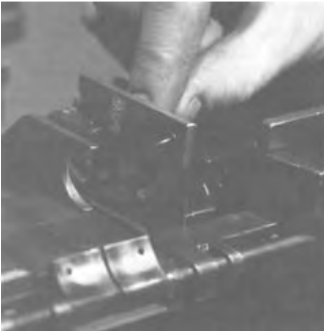
Figure 4-53. Inserting the Timing Gage.
