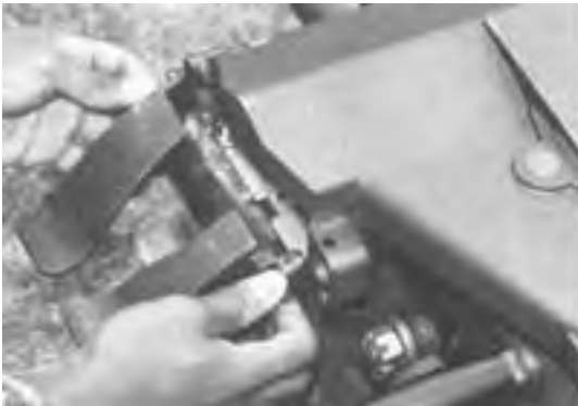
Figure 5-48. Attach Feed Throat to Feeder.
