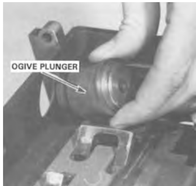
Figure 5-20. Removing the Ogive Plunger.
