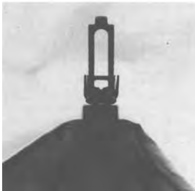
Figure 3-3. Rear Sight Assembly.
