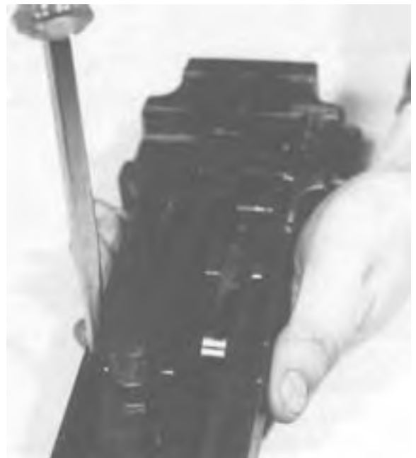
Figure 4-38. Removing the Belt Feed Lever.
