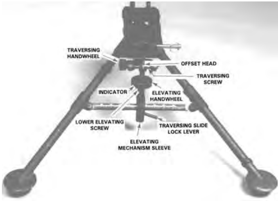
Figure 3-41. T&E Mechanism.
