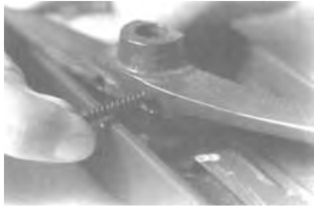
Figure 4-39. Removing the Shoulder Headless Pin and Spring.
