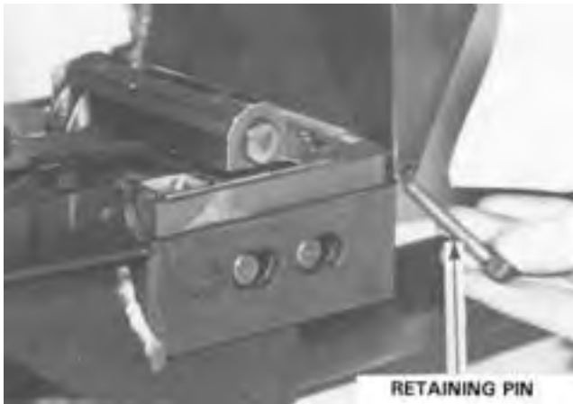
Figure 5-10. Removing the Feed Tray Cover Retaining Pin.
