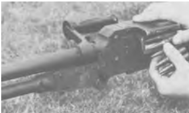
Figure 3-59. Loading, Cover Closed.
