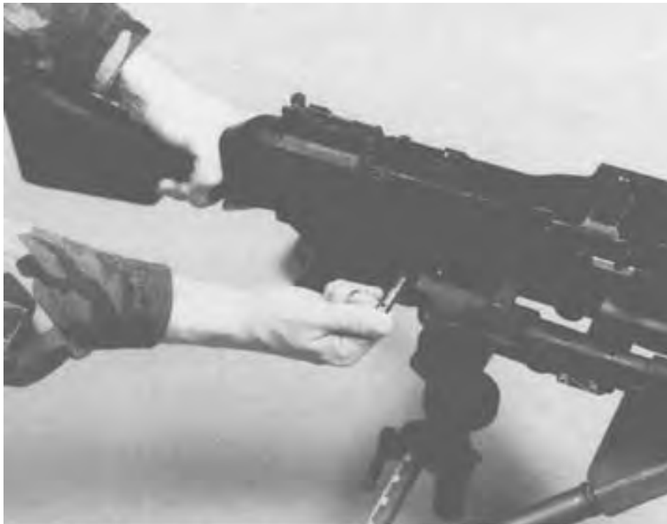
Step 2. Locking the Gun in Place with the Flex-mount's Rear Retaining Pin.
