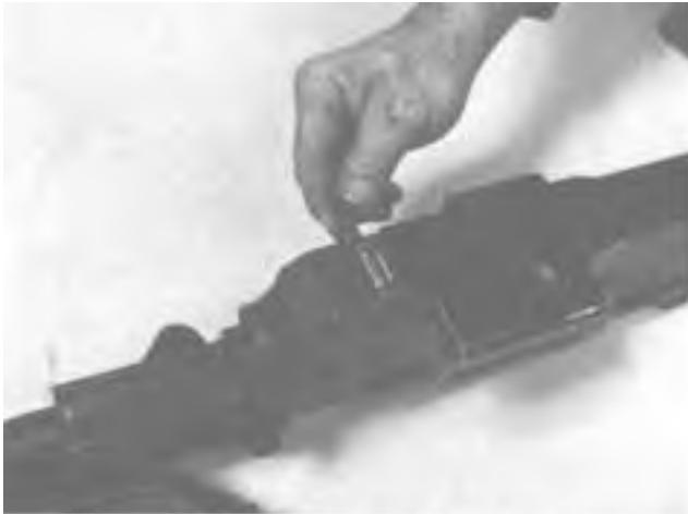
Step 1. Removing the Hinge Spring Pin.
