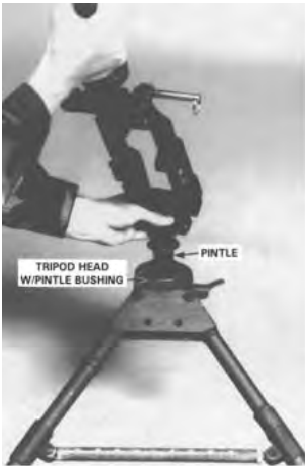
Step 1. Inserting the Pintle into Pintle Bushing.
