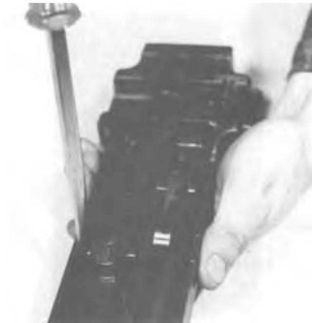
Figure 4-48. Snapping the Belt Feed Lever Lug to Seat the Shoulder Headless Pin.
