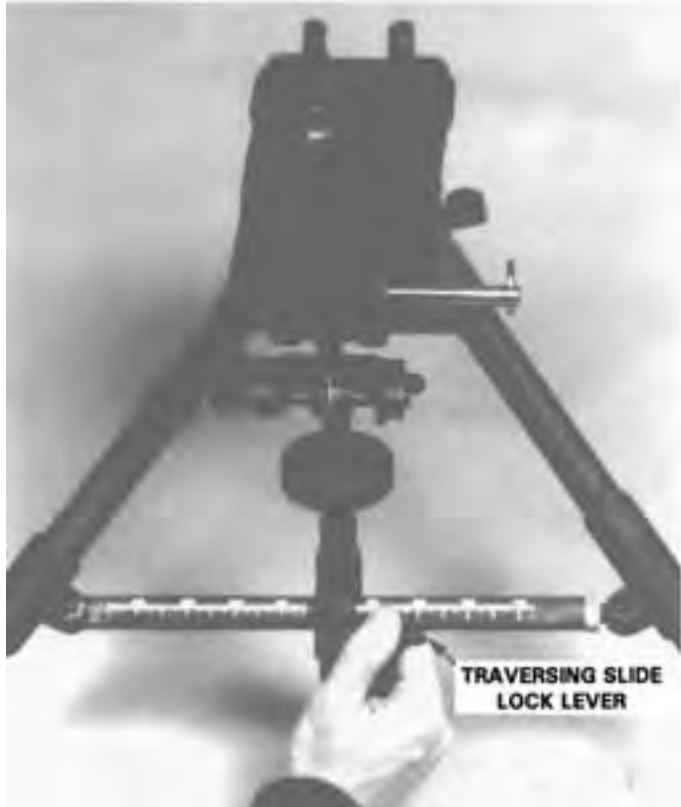
Figure 3-42. Attaching the Flex-mount to the Tripod—Continued.
