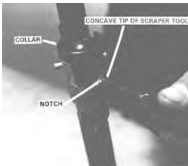
Step 1. Placement of the Scraper Tool.
