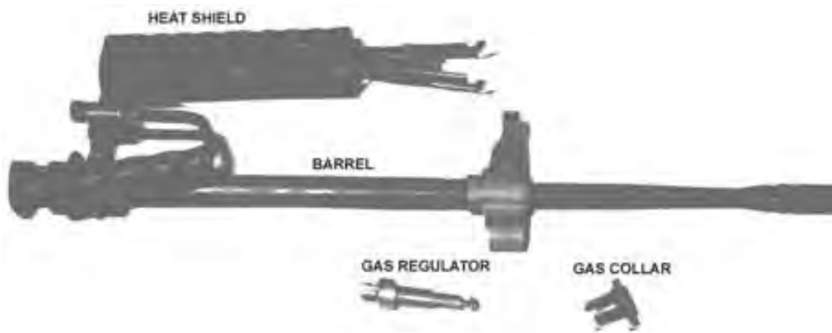
Figure 2-19. Barrel Group, Detail Disassembled.
