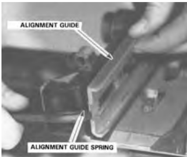
Figure 5-19. Removing the Alignment Guide Assembly.
