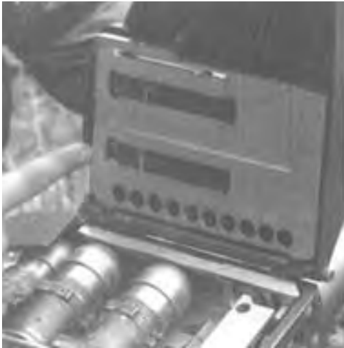
Figure 5-47. Moving Primary Drive Lever to the Right.
