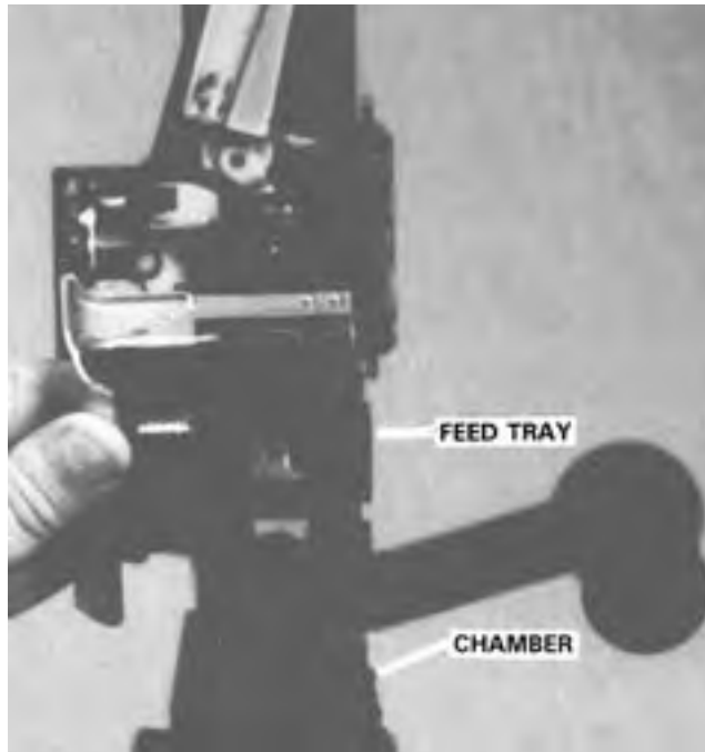
Figure 3-60. Inspecting the Chamber.
