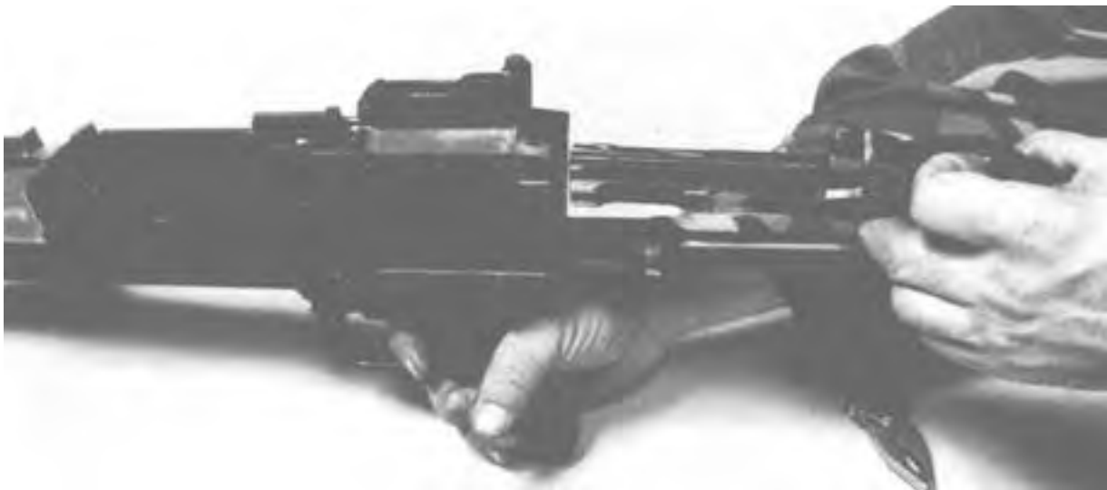
Figure 3-12. Replacing the Bolt and Operating Rod Assembly.
