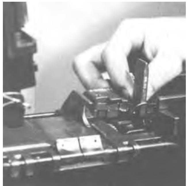
Figure 4-52. Inserting the Headspace Gage.
