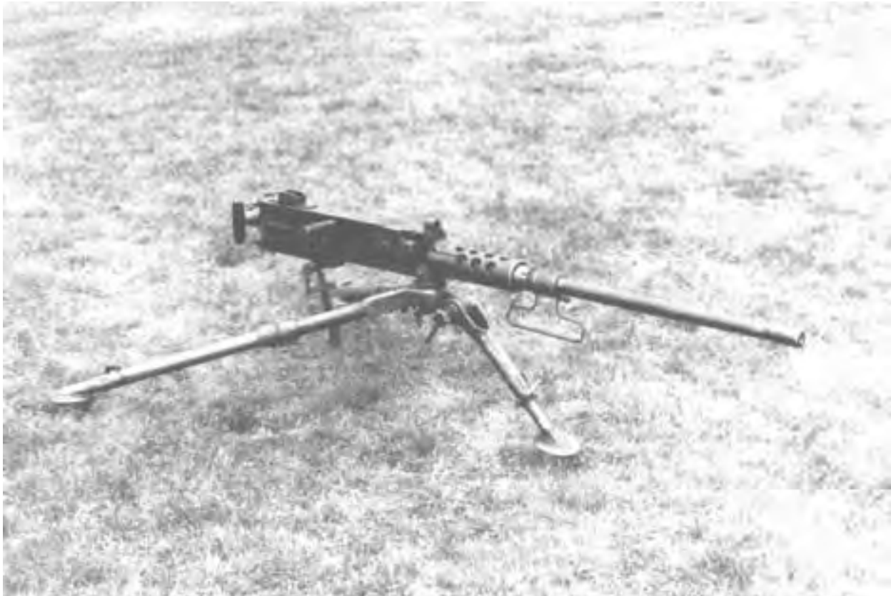
Figure 4-1. M2 .50 Cal on Tripod Mount, M3.
