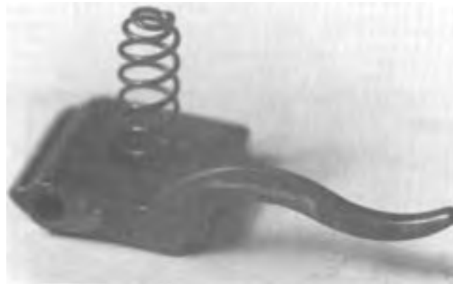
Figure 4-46. Seating the Belt Feed Pawl Spring (Left-Hand Feed).
