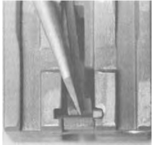
Figure 4-23. Prying the Sear Stop into the Center Recess.
