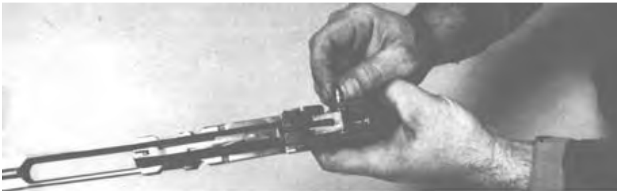
Step 1. Removing the Spring Loaded Pin.
