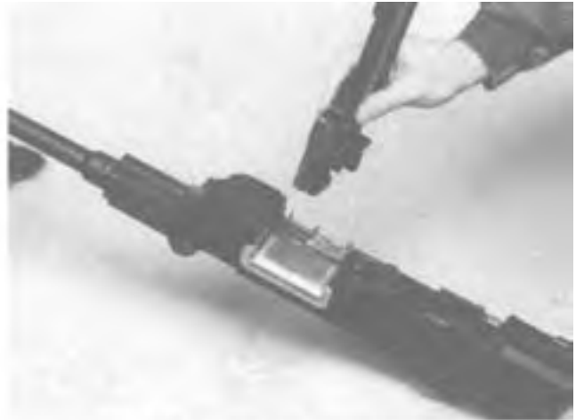
Step 2. Removing the Cover and Feed Tray.
