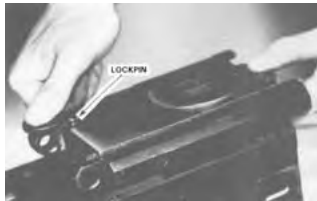
Figure 5-12. Lifting the Locking Pin.
