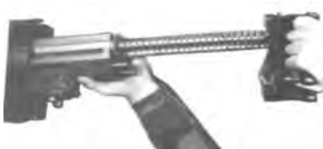
Figure 5-15. Depressing the Sear While Sliding the Bolt Assembly Forward.
