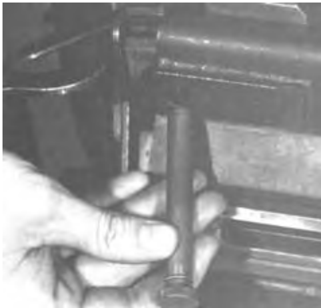
Figure 5-7. Removing the Bolt and Backplate Pin.
