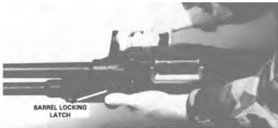
Step 1. Depressing the Barrel Locking Latch.
