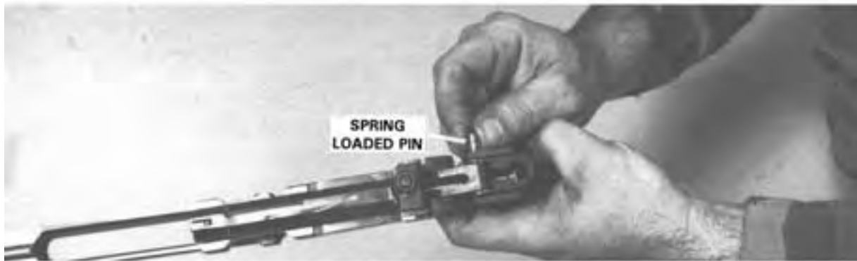
Step 2. Inserting the Spring Loaded Pin.
