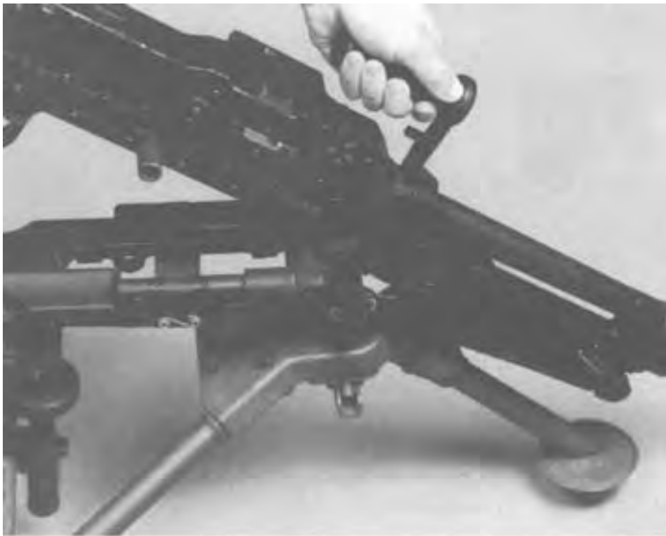
Step 1. Affixing the Gun to the Flex-mount's Forward Bushing.
