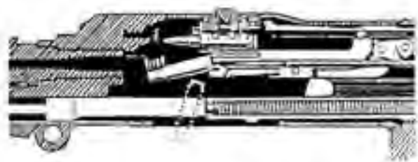
Figure 3-30. Extraction and Ejection.
