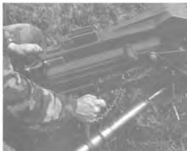
Figure 5-54. Placing and Securing the MK-19 into the Cradle.
