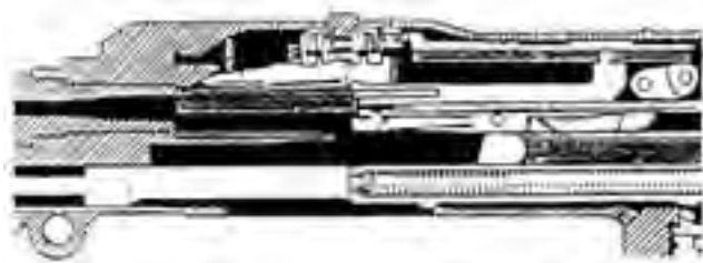
Figure 3-55. Firing From the Open Bolt Position.
