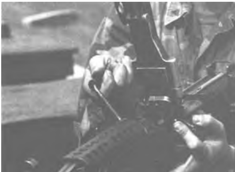
Figure 2-12. Replacing the Barrel Group.
