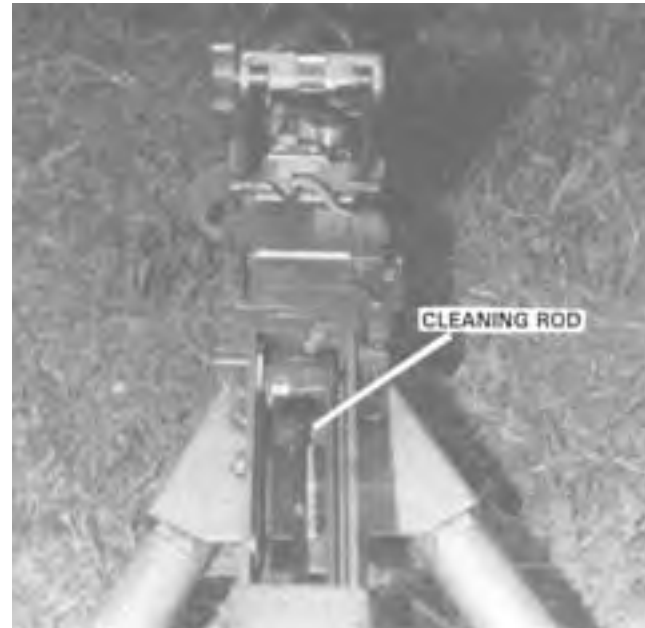
Figure 4-87. Clearing the Gun.
