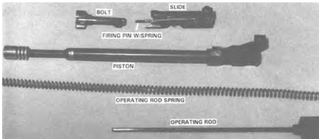
Figure 2-15. Operating Group, Detailed Disassembled.
