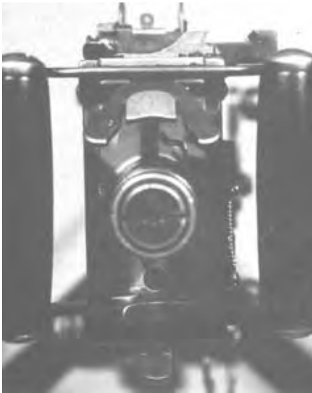
Figure 4-8. Bolt Latch Release Free of the Bolt Latch Release Lock.
