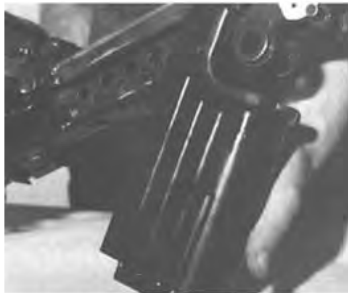
Step 2. Removing the Handguard.
