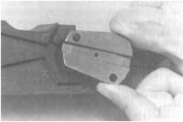
Figure 4-33. Replacing the Bolt Switch and Stud.
