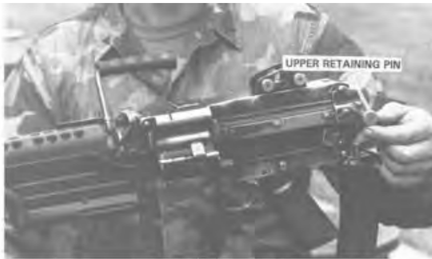
Step 1. Rotating the Buttstock Down.
