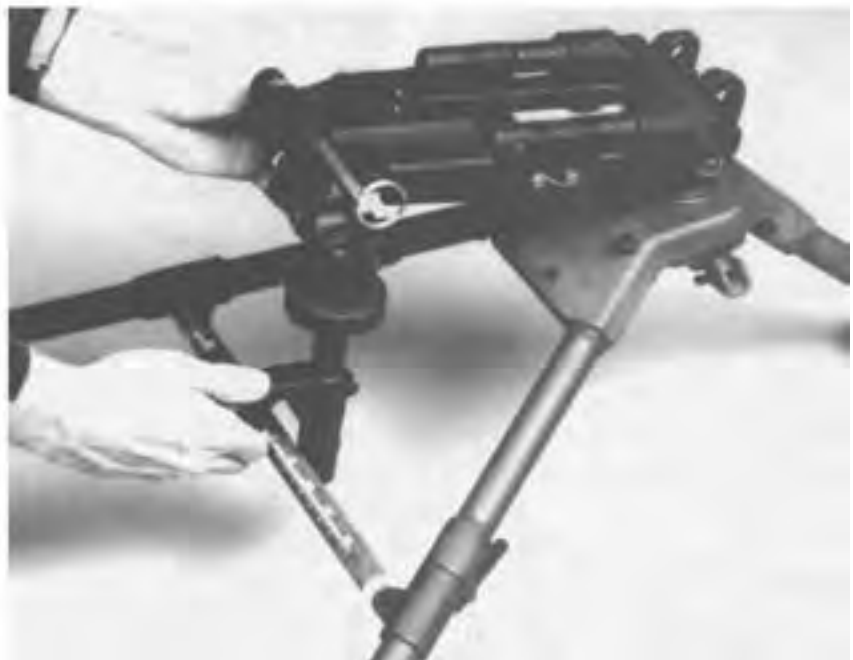
Figure 3-42. Attaching the Flex-mount to the Tripod.
